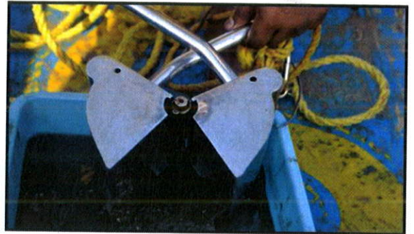
Sediment sample collected by using Van- Veen Grab
