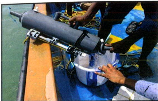
Sub-surface water sample collection by using Niskin water sampler
