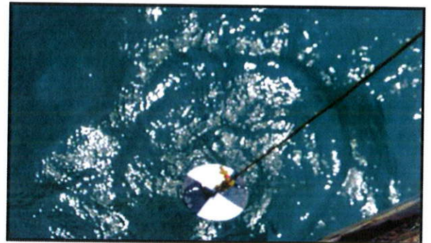
Vertical transparency measurement by using Secchi disc
