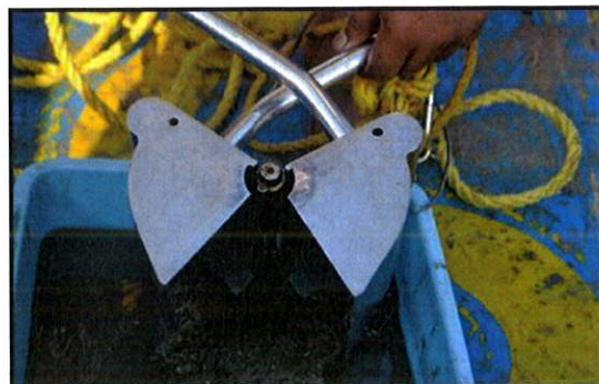
Sediment sample collected by using Van- Veen Grab
